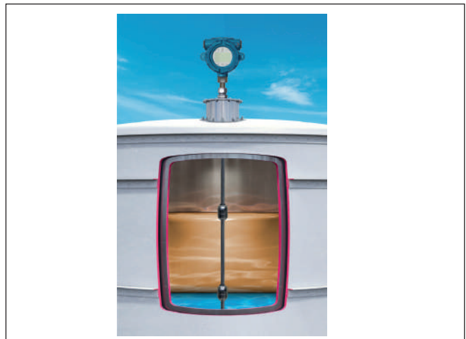
Fig. 2: Example of product and interface level measurement
