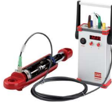
MH-Series Analog/PWM Tester, part no.: 280618
