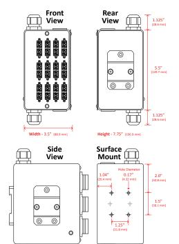
epth - with DIN-Rail mount 5.75" (146 mm
